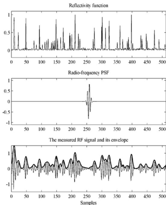
Figure 2. Simulated signals. Top: the generated reflectivity function. Middle: the generated PSF. Bottom: the resulted RF signal and its envelope.
