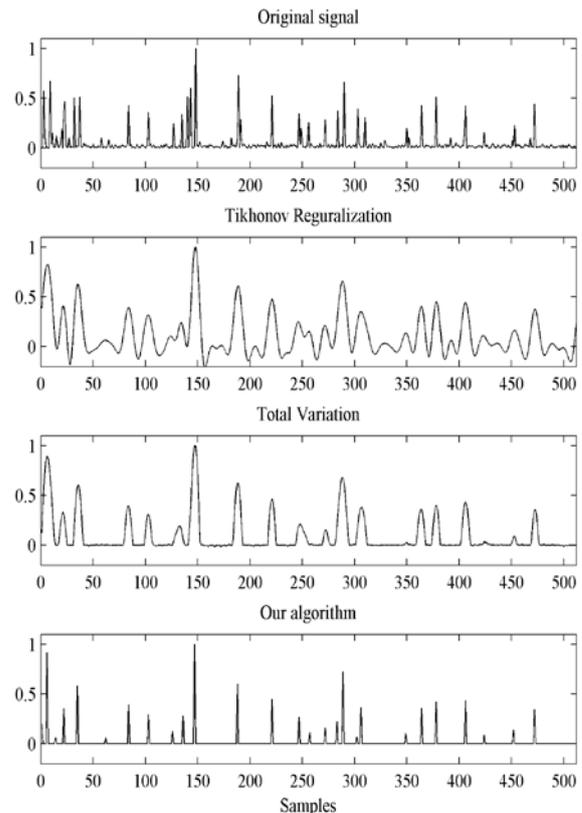
Figure 3. Top: original reflectivity function; Middle-top: results obtained with TkR; Middle-bottom: results obtained with TV; Bottom: results obtained with our algorithm.
