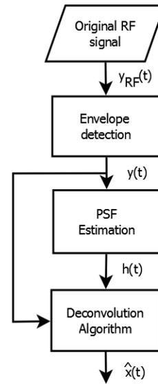
Figure 1. The steps of the algorithm implementation.
