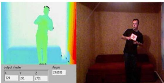
Figure 5. RGB and depth image of the Kinect sensor, and the measured position and orientation of the box
