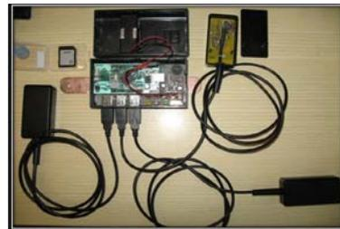
Figure 1. MMA7260QT 3-axis accelerometer sensor AT MEGA 128 microcontroller USB connectors MMC card for data storage
