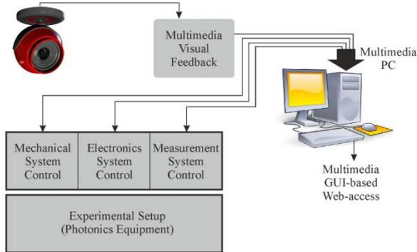
Figure 3. Web-based multimedia laboratory system.
