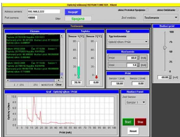
Figure 7. Main control window for the Measurement of the laboratory refractometer.
