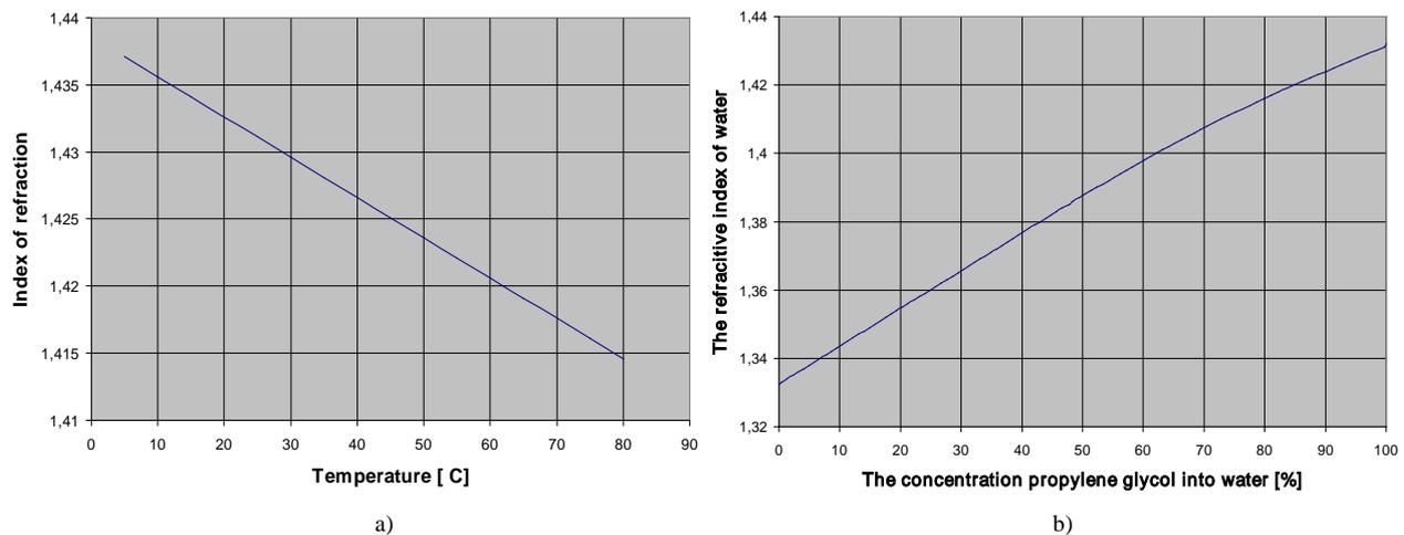
Figure 8. The refractive index of a) the propylene glycol vs. temperature ( $^{\circ}\text{C}$ ) and b) the water vs. propylene glycol concentration.
