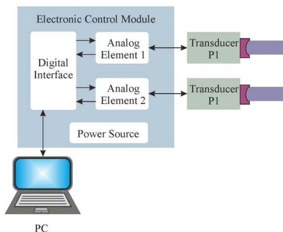
Figure 2. Block scheme of the laboratory fiber optic refractometer equipment.
