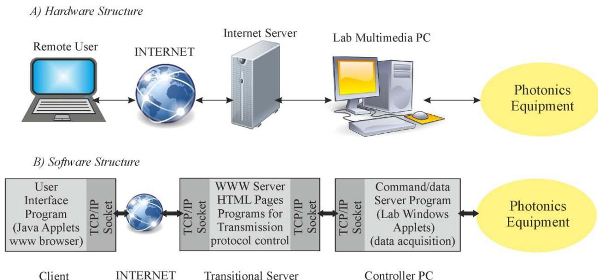
Figure 1. Web-controlled laboratory architecture.
