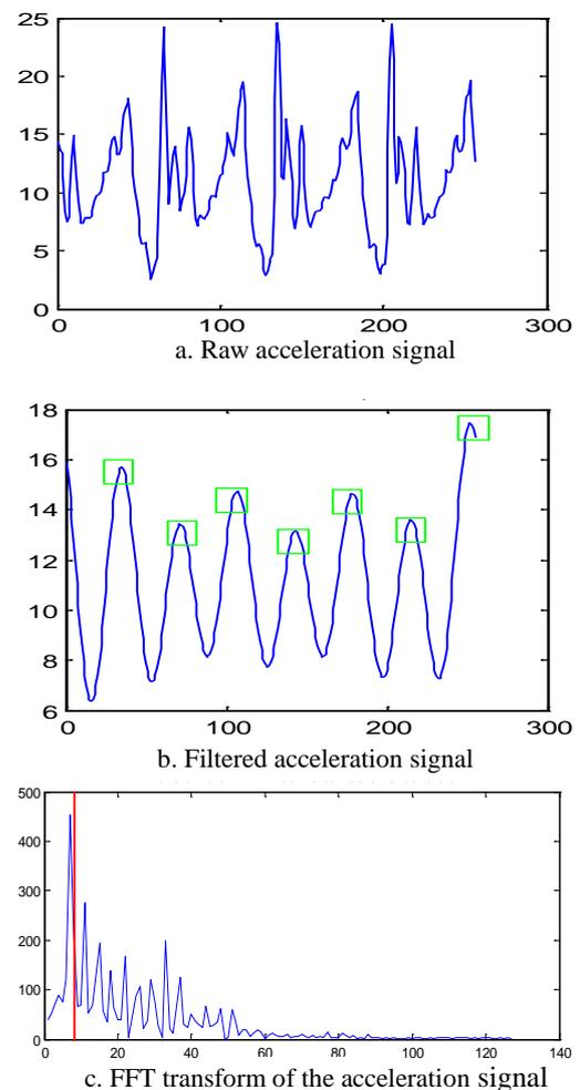
Figure 2. Processing of acceleration signals
