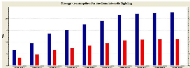
Figure 12. Energy consumption for 500 lux with movement detection, 8 humans
