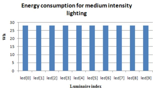
Figure 6. Energy consumption for 500 lux lighting
