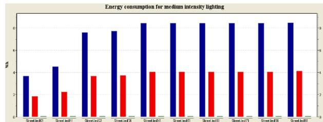
Figure 10. Energy consumption for 500 lux with movement detection, 2 humans
