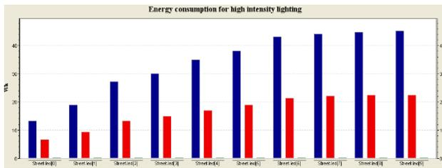
Figure 11. Energy consumption for 1 lux with movement detection, 8 humans
