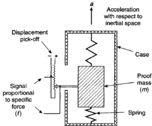
Figure 1. A simple accelerometer [5]
