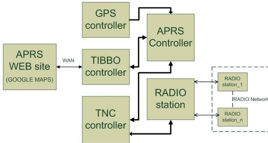
Figure 1. APRS node controller project structure
