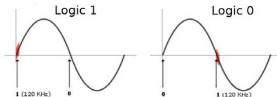
Figure 2. X10 protocol encoding
