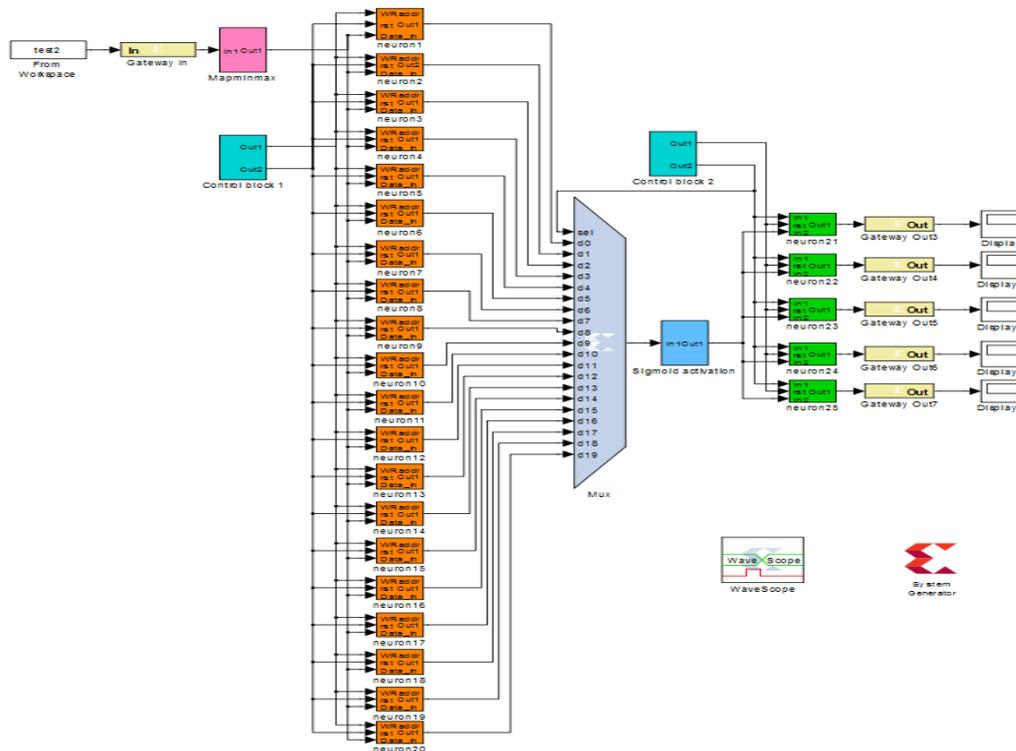
Figure 6. Neural network model in System Generator
