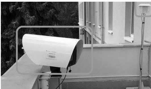
Fig. 1. Free Space Optics head (model Light Point – Flight Strata 155) on the left. Fog sensor with ability of measuring different atmosphere parameters (temperature, humidity, pressure, altitude, lwc). This setup is located within a campus of Technical University of Kosice (Vysokoskolska 4).
