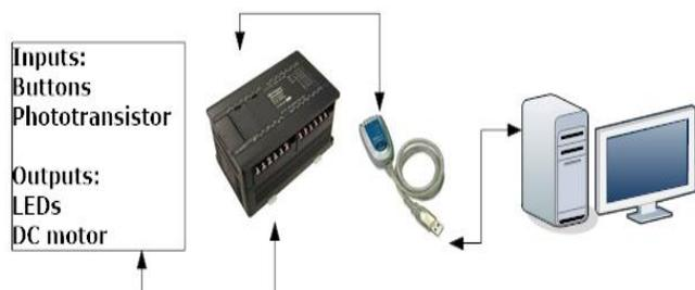
Fig. 3 – Schematic of the Control Platform
