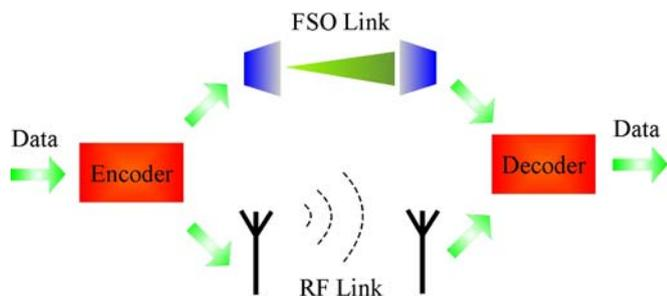
Fig. 2. Schema of the soft switching.
