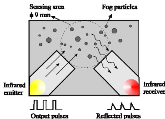
Fig. 4. Principle of measuring density of fog.
