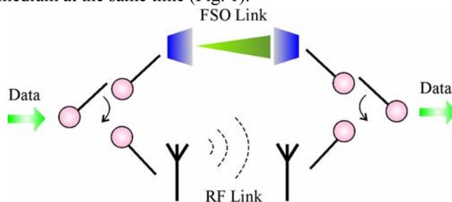
Fig. 1. Schema of the hard switching.
