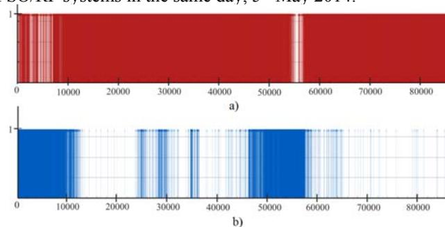
Fig. 6. Activity diagram of Hybrid FSO/RF system, 5<sup>th</sup> May 2014; a) FSO activity, b) RF activity for 150 m.
