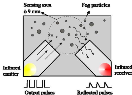
Fig. 4. Principle of measuring density of fog.
