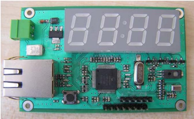
Fig. 4. Our prototype DSN-PC station [9].
