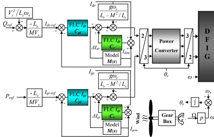
Figure 6. Bloc diagram of the adaptive fuzzy logic control of the DFIG.
