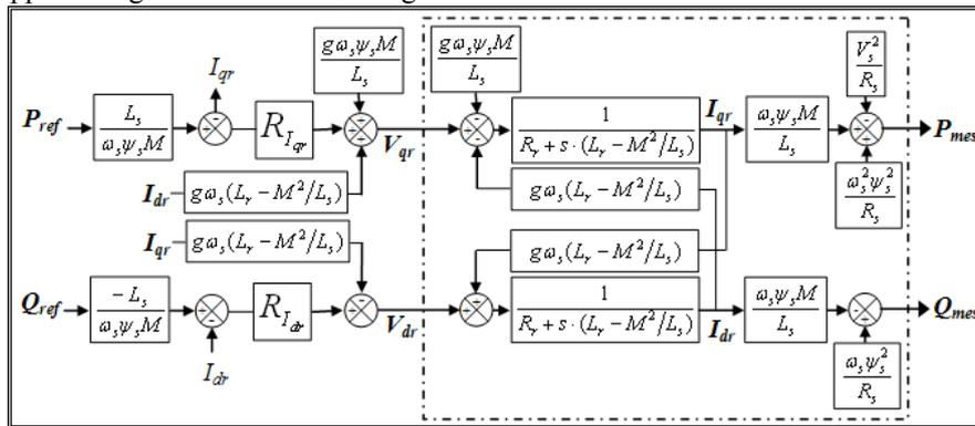
Figure 1. Power control of DFIG.
