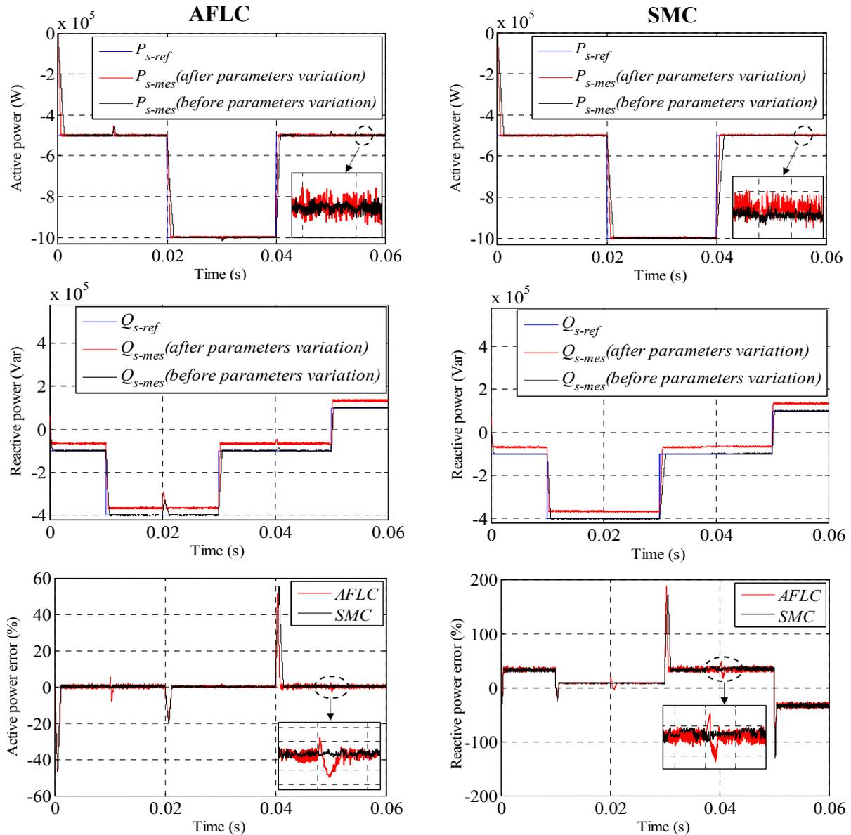
Figure 9. Effect of machine's parameters variation on the DFIG control.
