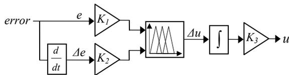
Figure 3. Block diagram of fuzzy logic controller.
