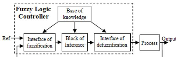
Figure 2. Structure of fuzzy logic controller.
